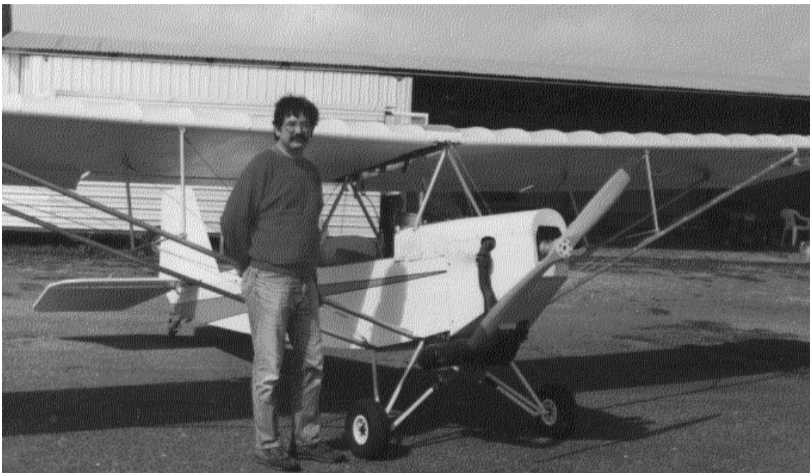
Charlie Ramos has one of the oldest ChuckBirds - now 13 years old! This bird has a 50 hp 2-stroke engine and flaps. Charlie likes to drop the flaps and "park" a few hundred feet over the airport.
