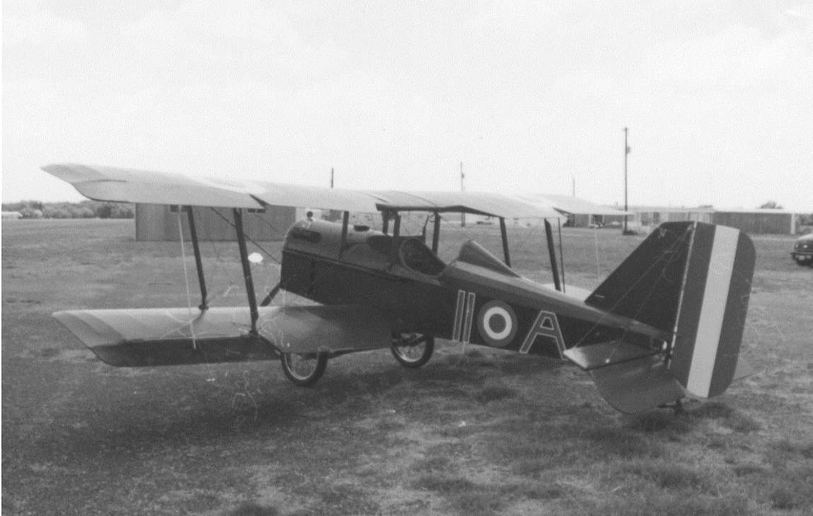
SE-5 replica with a 3-cylinder Geo engine and a Rotax gearbox
