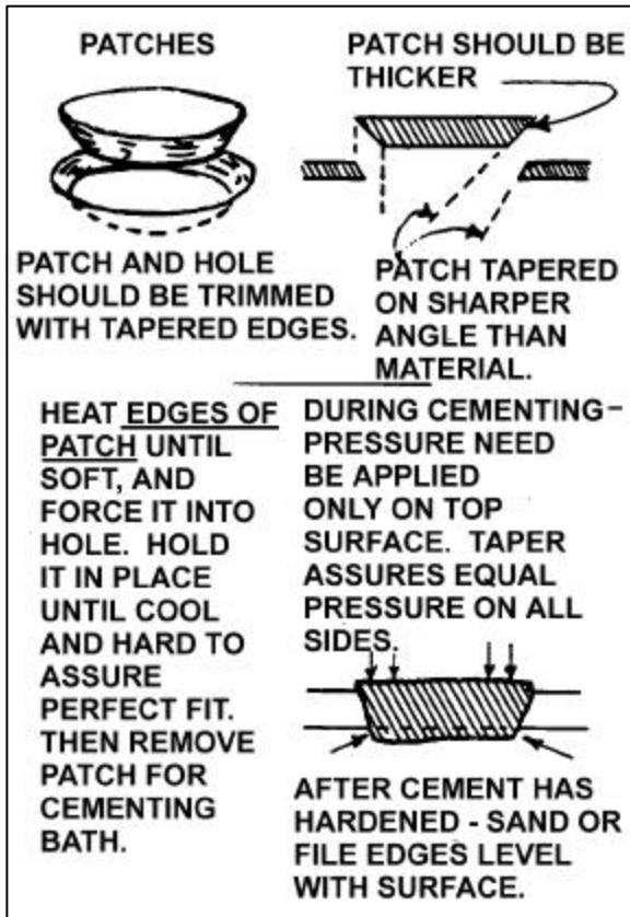
FIGURE 3-23. Plug patch repair.
